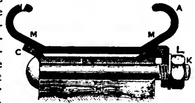
CROSS SECTION OF VINET RIM.
